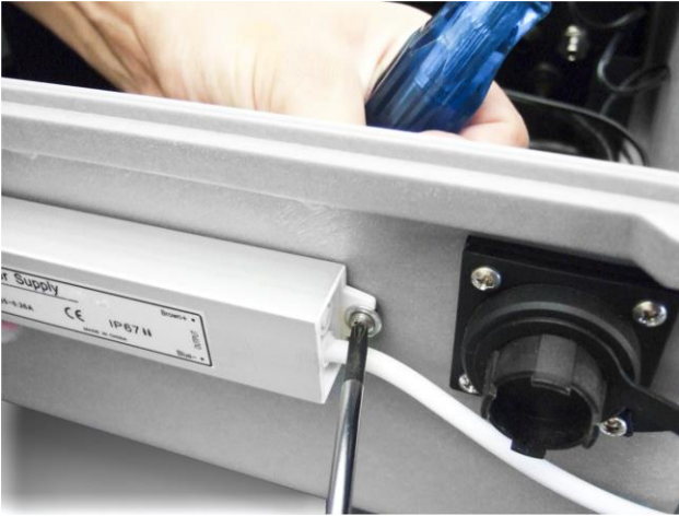
Figure 24: Attach the Adapter to the Enclosure
