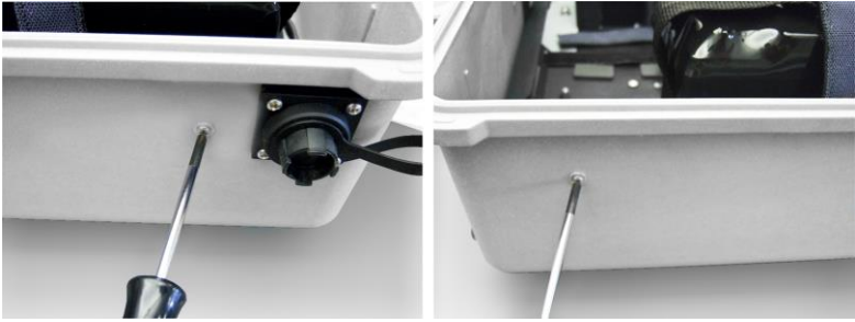
Figure 23: Remove the Adapter Mounting Screws
