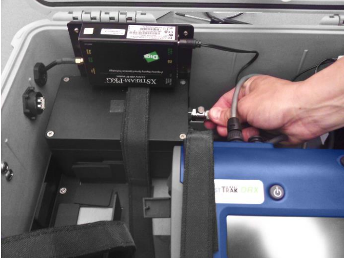
Figure 31: Connect External Pump Flow Tube
