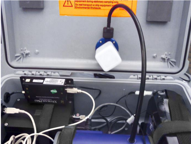
Figure 35: Connect Sample Tubing
