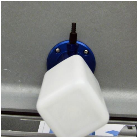
Figure 7: Install the Water Trap Bottle
