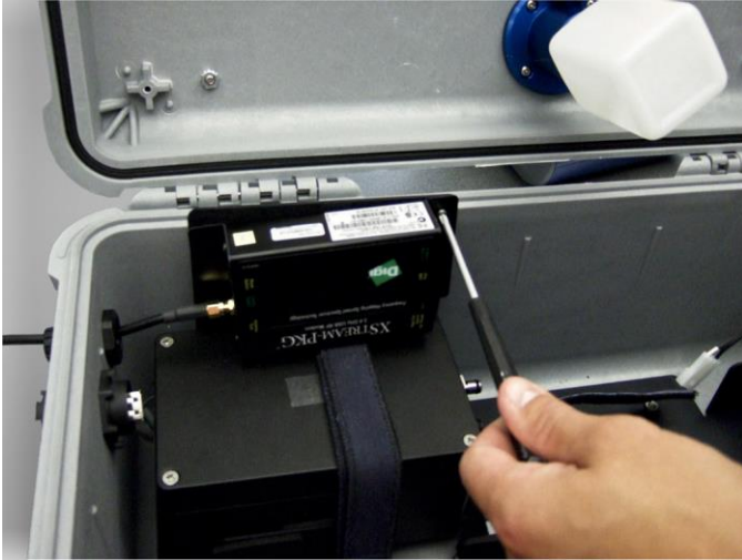
Figure 13: Attach Radio Modem to Bracket
