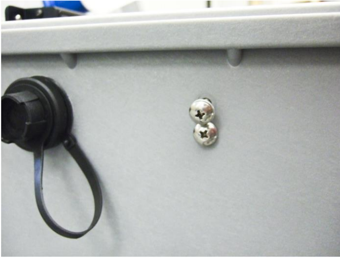
Figure 15: Remove Two Screws to Secure Antenna
