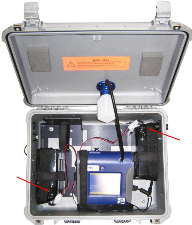
Figure 22: Install the Dual Battery Pack System
