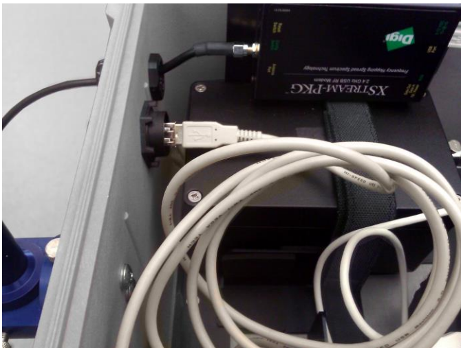
Figure 34: Connect USB Cable for Pass-through
