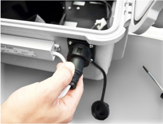
Figure 25: Connect Adapter DC Cable to Enclosure
