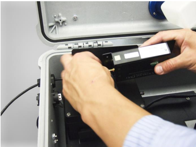
Figure 12: Attach Antenna and Cable to Radio Modem
