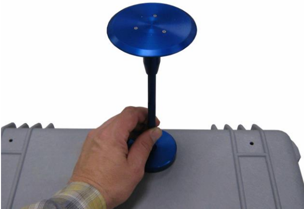
Figure 3: Thread the Inlet into the Inlet Ring
