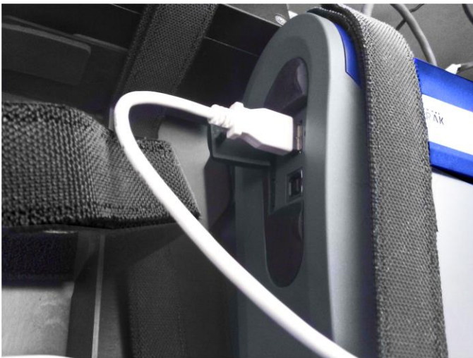
Figure 32: Connect Square (B-type) USB Cable to Radio Modem
