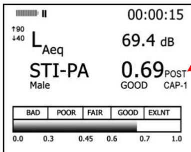
Figure 6-27: Post CAP-1 applied during STI-PA test
