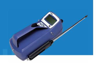
The TSI's P-Trak® Ultrafine Particle Counter (UPC) 8525 is an ideal instrument for measuring workplace ultrafine particulate levels, as well as helping eliminate indoor air quality (IAQ) problems.
